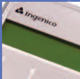
2 lines of 16 characters display eliminates the need for message scrolling
